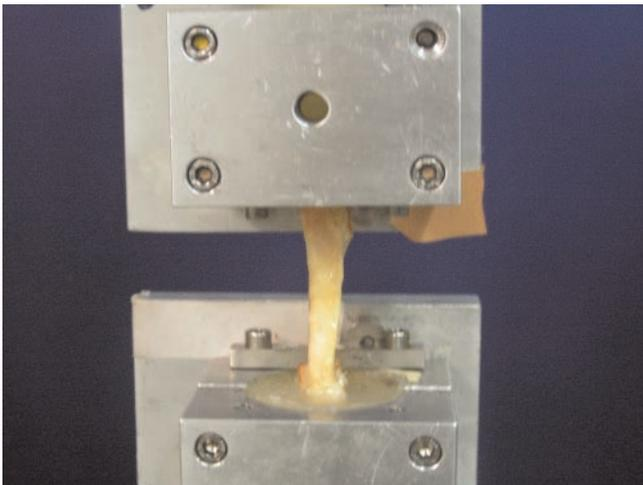
**Figure 3.** Testing setup with the graft embedded in polymethylmethacrylate and fixed in aluminum clamps for mechanical testing.
